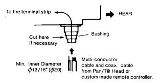
Pass the cables through the wiring hole.
