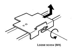
Fix the camera mounting plate on the bottom of the camera using two screws.
