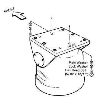
Be sure to align the camera direction and front direction of Pan/Tilt Head.
